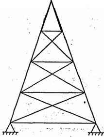
What is the total degree of indeterminacy (both internal and external) of the triangular planar truss shown in the figure above?
