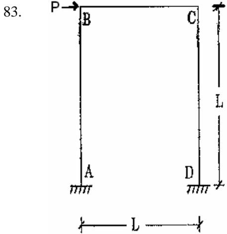
What is the shear equation in slope deflection method for the portal frame shown above?
