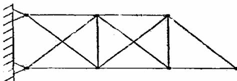
What is the total degree of indeterminacy (both internal and external) of the cantilever plane truss shown in the above figure?
