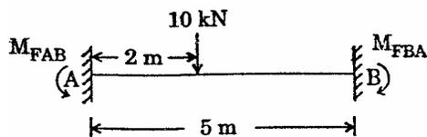
A fixed beam AB, of constant  $EI$ , shown in the above figure, supports a concentrated load of 10 kN. What is the fixed end-moment  $M_{FAB}$  at support A?
