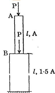
A stepped column carries loads as shown above. What is the maximum normal stress in the column at B in the larger diameter column?
