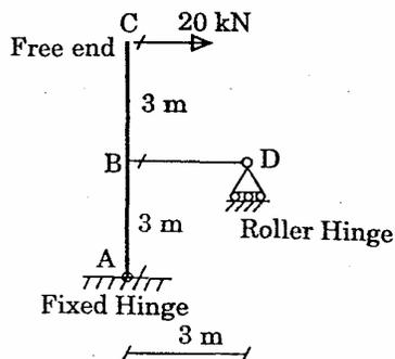
What is the reaction at the support D of the rigid-jointed structure shown above?
