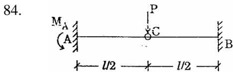
The fixed beam AB has hinge C at mid span. A concentrated load P is applied at C. What is the fixed end moment  $M_A$ ?
