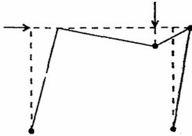
A portal frame has a collapse mechanism as shown above. What is the type?
