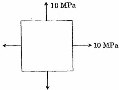
What is the diameter of Mohr's circle of stress for the state of stress shown above?
