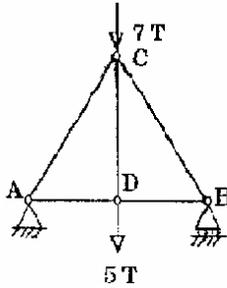
What is the force in the vertical member CD of the pin-jointed frame shown above?
