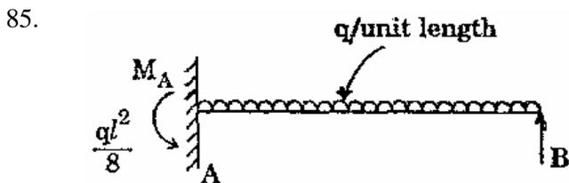
The propped cantilever AB carries a uniformly distributed load of  $q$ /unit length. In this condition the moment reaction
