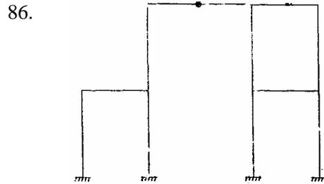
What is the static indeterminacy for the frame shown above?
