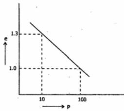
The virgin compression curve for a soil is shown in the figure above. What is the compression index of the soil ?
