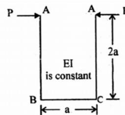
In the structure shown in the figure above, what is the distance through which the points A move towards each other?
