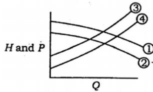
The performance of a centrifugal pump [H and P vs. Q] is typically shown in the figure with four curves numbered 1, 2, 3 and 4. which one of the following is correct?
