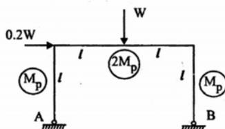
Collapse moment for the frame shown above has been worked out as  $M_p = Wl/5$ .
