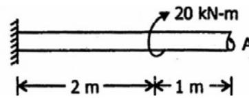
A circular shaft of diameter 30 mm having shear modulus  $G = 80$  GPa is subjected to moment as shown above.
