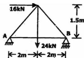
What are the magnitudes of horizontal and vertical support reactions, respectively at support A of the frame shown above ?
