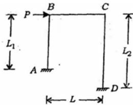
The shear equation for the portal frame shown in the above figure will be
