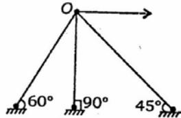
What is the most appropriate method for analysis of a skeletal plane frame shown in the figure above?
