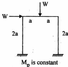
What is the ultimate load for the frame shown in the figure above ?
