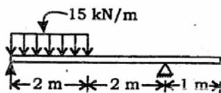
At what distance from left support of the above beam, is the shear force zero?
