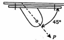
Four bolts share the load  $P$  as shown in the figure above. The shear strength of bolt is 30 kN and tension strength of bolt is 40 kN.
