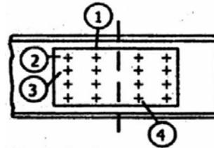
Which one of the bolts in a web splices of a plate girder as shown in the figure is stressed maximum?
