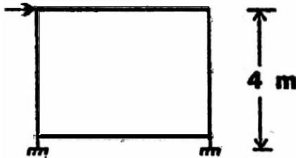
An industrial portal frame shown has weak floor beams. What is the effective length of column ?
