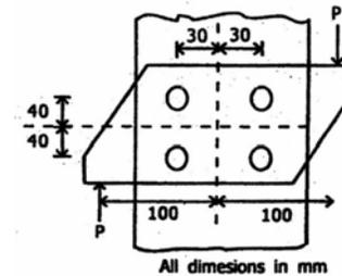
A bracket has been attached to flange of a column as shown in the figure. What is the maximum force in the bolt ?
