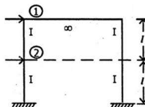
The beams in the two storey frame shown in the figure above have a cross section such that the flexural rigidity may be considered infinite. Which among the following is the stiffness matrix for the structure in respect of the global coordinates 1 and 2?
