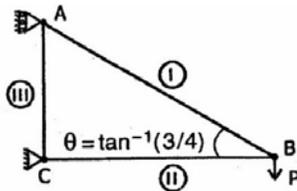
A cantilever truss carries a concentrated load P as shown in the figure above. What are the magnitudes of axial forces in the members I, II and III, respectively?
