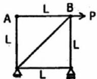
What is the force in number AB of the pin-jointed frame as shown above ?
