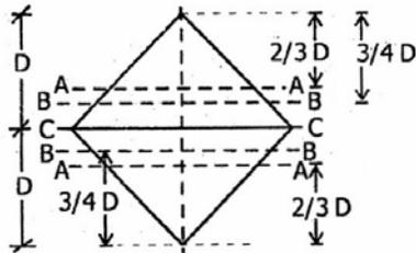
A beam of square cross section is placed horizontally with one diagonal horizontal as shown in the figure above. It is subjected to a vertical shear force acting along the depth of the cross section. Maximum shear stress across the depth of cross section occurs at a depth  $x$  from the top. What is the value of  $x$ ?
