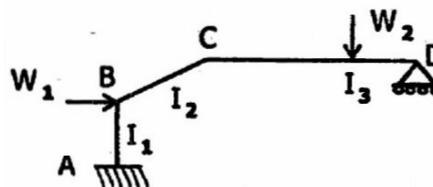
The rigid plane frame ABCD has to be analysed by slope deflection method. What is the number of unknown displacements / rotations for the frame as shown in the figure given above?
