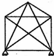
What is the degree of static indeterminacy of the plane structure as shown in the figure above?
