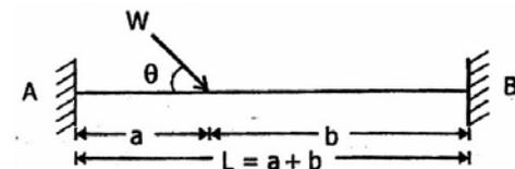
For the fixed beam as shown in the figure above, what is the fixed end moment at A for the given loading?
