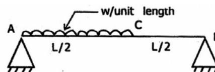
A simply supported beam AB has span  $L$  as shown in the figure above, Point C is the mid—span of the beam. It is subjected to u.d.l.  $w/\text{unit length}$ , in the portion A to C. Which of the following are the SFD and BMD for the beam ?
