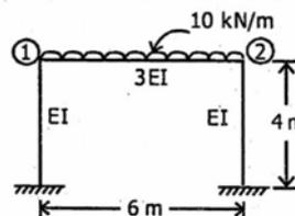
Considering only flexural deformations, which is the stiffness matrix for the plane frame shown in the figure given above?
