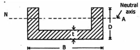
A horizontal beam shown in the figure given above is subjected to transverse loading. Which one of the following diagrams represents the distribution of shear force along the cross-section?
