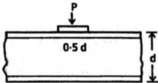
A plate girder of depth  $d$  bears a concentrated load  $P$  through a distribution plate of width  $0.5d$  as shown in the figure. If the maximum allowable critical buckling stress is calculated as  $f$ , what is the value of  $P$ ? Web plate thickness =  $t$
