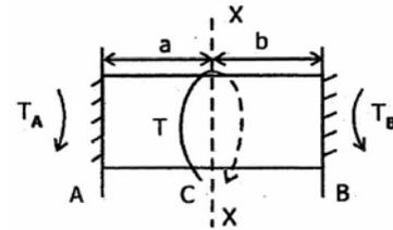
For the circular shaft AB, as shown in the figure above, a torque 'T' is applied at the section XX at C, such that  $b/a = 1.5$ . The shaft is uniform in section. What is the ratio of  $T_A/T_B$ ?
