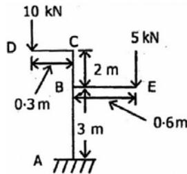
Which one of the following is the bending moment diagram for the vertical cantilever beam loaded as shown in the figure above?
