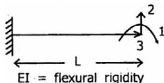
What is the stiffness matrix for a prismatic cantilever with coordinates as shown in figure ?
