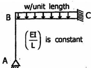
What is the ratio of magnitudes of moments in the member BC at the ends B and C in the figure given above?
