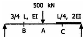
A load 500 kN applied at point A, as shown in the figure above, produces a vertical deflection at P and C of the beam as  $\Delta_b = 10$  mm and  $\Delta_b = 15$  mm respectively. What is the deflection at A when loads of 100 kN and 300 kN are applied at B and C. respectively?
