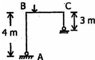
For the frame as shown in the figure above, the final end moment MDC has been calculated as  $-40$  kNm. What is the end moment MCD?
