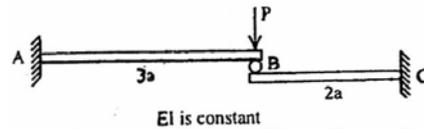
The free end of a cantilever beam is supported by the free end of another cantilever beam using a roller as shown in the figure given above. What is the deflection at the roller support B?
