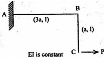
What is the vertical displacement at the point C of the structure shown in the figure given above?
