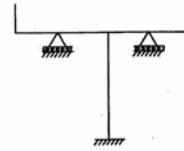
What is the degree of indeterminacy of the frame shown in the figure given above?
