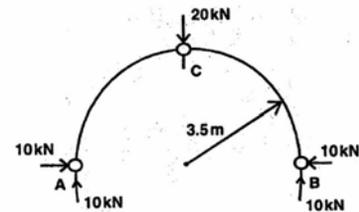
A three-hinged loaded semicircular arch ACB is shown in the figure given above. What is the shearing force at the hinge C?
