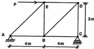
What is the ratio of the forces in the members AB, BE and AE of the pin-jointed truss shown in the figure given above?
