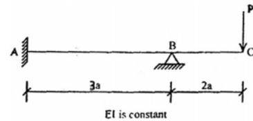
In the propped cantilever shown in the figure given above, what are the values of the bending moment and shear force at the support A?
