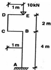
What is the bending moment at A for the bent column shown in the figure given above?
