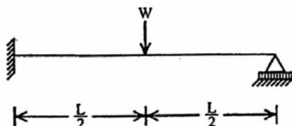
For the propped cantilever beam shown in the figure given above, the plastic moment
