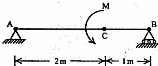
Couple M is applied at C on a simply supported beam AB. What is the maximum shear force for the beam?
