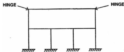
What is the total degree of indeterminacy, both internal and external of the plane frame shown above?
