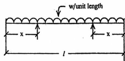
A uniform beam of span  $l$  carries a uniformly distributed load  $w$  per unit length as shown in the figure given above. The supports are at a distance of  $x$  from either end. What is the condition for the maximum bending moment in the beam to be as small as possible?
