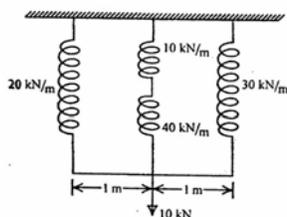
What is the equivalent spring stiffness for the system of springs shown in the figure given above?
