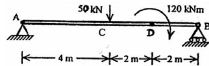
The beam shown in the figure given above is subjected to concentrated load and clockwise couple.
