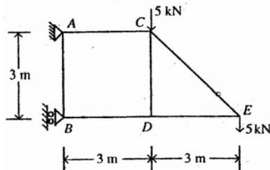
The diagram above shows a truss subjected to loading as indicated. What is the force induced in the member AB?
