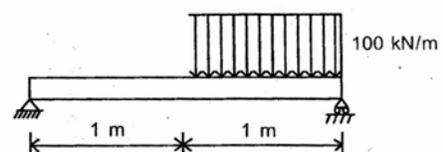
The above diagram shows a simply supported beam with load. Which one of the following diagrams is the shear force diagram for this beam ?
