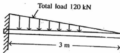
What are the support reactions at the fixed end of the cantilever beam shown in the above diagram?
