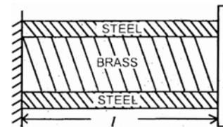
A brass bar of solid section is encased in a steel tube as shown in the above diagram
