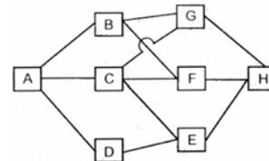
Consider the above AOA diagram. What is the minimum number of dummy arrows required for conversion into AOA diagram ?
