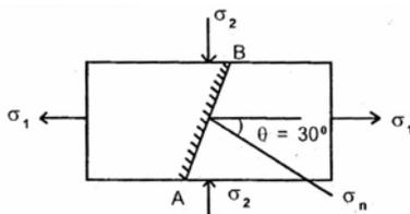
In a piece of stressed material, the principle stress are  $\sigma_1 = 3.0 \text{ kN/m}^2$  tensile and  $\sigma_2 = 7.0 \text{ kN/m}^2$  compressive as shown in the above diagram. The line of action of the tensile stress makes an angle  $\theta = 30^\circ$  to the normal to the plane AB. What is the normal stress  $\sigma_n$  ?
