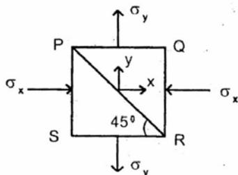
A thin wooden plate PQRS is made by gluing two pieces of wood along PR as shown in the above diagram.
