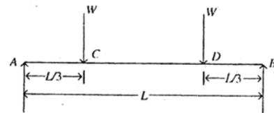
Consider the simply supported beam AB subjected to the point loads of equal magnitude as shown in the above diagram.
