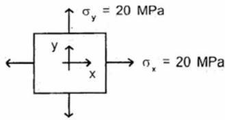
For the plane stress situation shown in the above diagram, what is the maximum shear stress ?
