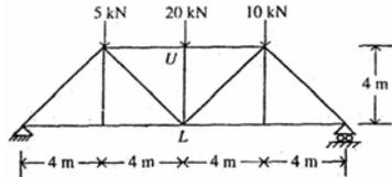
The diagram above shows a plane truss. What is the force in vertical member UL of the truss ?
