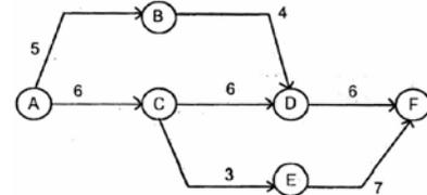
A network of seven activities is shown in the diagram given above. The respective activity durations are shown beside the arrows. Which one of the following is the total float in AB, the total float in CE and free float in EF, respectively ?
