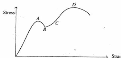
The stress strain diagram for mild steel subjected to tensile load is given above.
