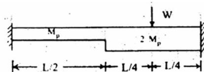
At the point of collapse, the value of load W will be
