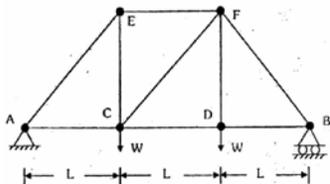
34. In the truss shown in the figure given above, which one of the following members has no force induced in it ?
