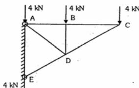
The force in the member BD of the truss shown in the figure given above is
