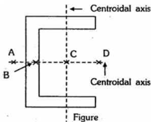
In the symmetrical channel section shown in the figure, which point is likely to be the shear center ?
