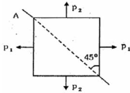
$p_1$  and  $p_2$  are two equal tensile principal stresses. On the plane AB inclined at  $45^\circ$  to the plane of  $p_1$
