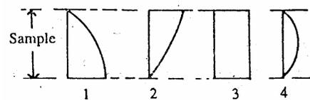
Excess pore pressure distribution within the thickness of a soil sample tested in oedometry sometime after loading is shown in the above figures labeled 1, 2, 3 and 4. Which one of these figures, refers to a situation where the operator forgot to put
