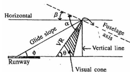
In the above figure shown, “cockpit cutoff angle” is the angle labelled
