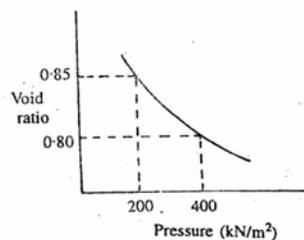
The e-p curve for a soil is shown in the above figure. The coefficient of compressibility (in  $\text{m}^2/\text{kN}$ ) of the soil is
