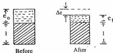
The figure given above shown the state of a sample of clay before and after consolidation. Based on these figures, the settlement of a clay layer of initial thickness H will be
