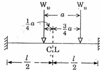
Which one of the following sketches gives a probable failure mechanism of this beam under plastic analysis ?
