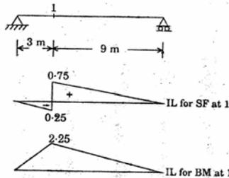
The values of the shear force and bending moment at section '1' due to a concentrated load of 20 kN placed at mid-span will be
