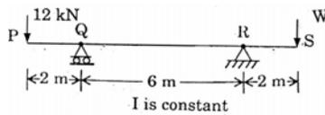
The magnitude of reaction at R will be zero if the value of load 'W' is
